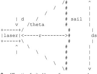
$\begin{aligned} \theta &= \text{ diffraction limited beam divergence angle} \\ r &= \text{ separation between laser and sail} \\ d_{\text{s}} &= \text{ sail diameter} \\ d &= \text{ laser transmitter aperture} \end{aligned}$
